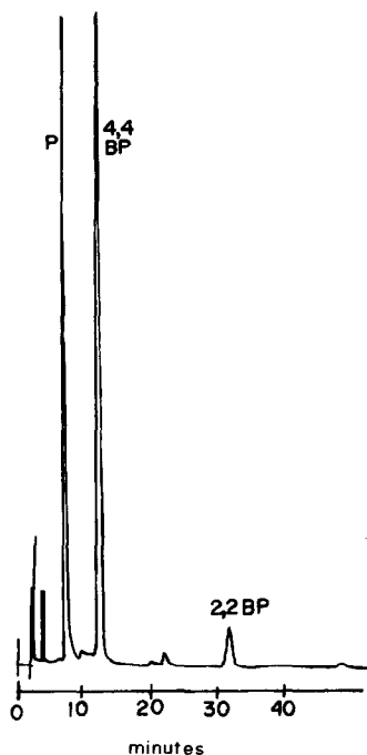
Figure 6 Peroxidase metabolism of phenol. Detection of 4,4'-biphenol (4,4-BP) and 2,2'-biphenol (2,2-BP). E = +1.00 V. Chromatographic conditions given in text. P = phenol.
